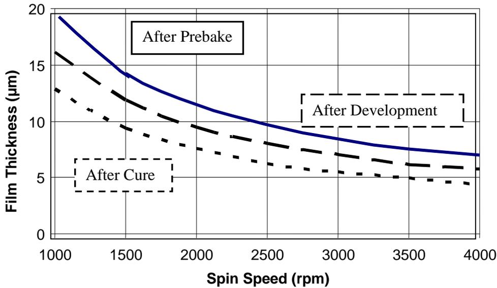
Table 1 illustrates the range of coating thicknesses obtainable from HD-8820. This is a guide, as different substrates, wafer size, surface topography, cleanroom conditions, softbake conditions, development times and cure conditions will affect final cured film thickness.
