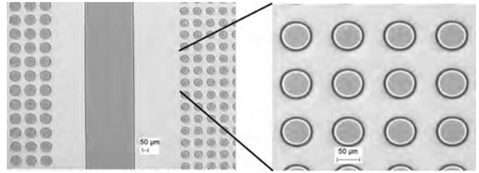
Fig. 13. Patterned HD-7010 film after bonding: (a) arrays of 80 and 60 μm vias with street (left), (b) 60 μm vias (right).
