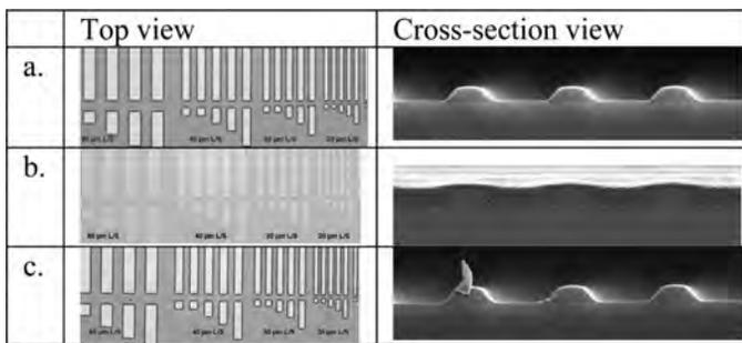
Fig. 10. Selective removal of HD-3007: (a) patterned film of HD-4004, (b) cured HD-3007 coated over the patterned film, and (c) HD-4004 pattern after removal of HD-3007 with EKC800. Top views of 20-60  $\mu\text{m}$  L/S, cross-section view of 6  $\mu\text{m}$  L/S.
