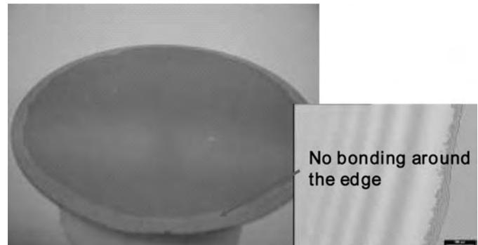
Fig. 2. Incomplete bonding of HD-3007 at  $200^\circ\text{C}$ .
