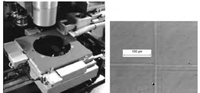
Fig. 8. UV Laser de-bonding: (left) wafer on precision stage below the laser, and (right) residue from overlapping pulses on the carrier, after debonding.
