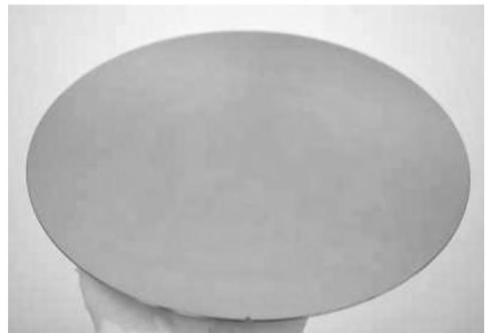
Fig. 3. Complete bonding of HD-3007 at  $300^\circ\text{C}$ .
